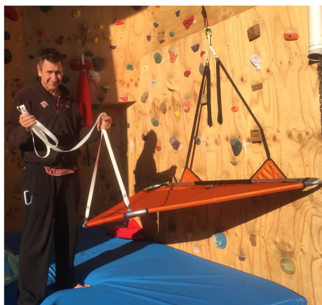
First step--unclip airside straps and stuff in bag
